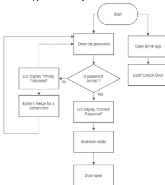
Fig. 4 IoT Smart Door using Keypad and Blynk Process.
